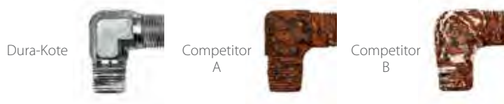
Corrosion comparison after 650 hours of exposure to salt spray testing.
